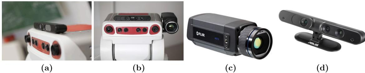
**Fig. 3.8:** PR2 mounted additional sensors: Asus Xtion Pro Live (a,d) and Flir A615 thermal camera (b,c)
