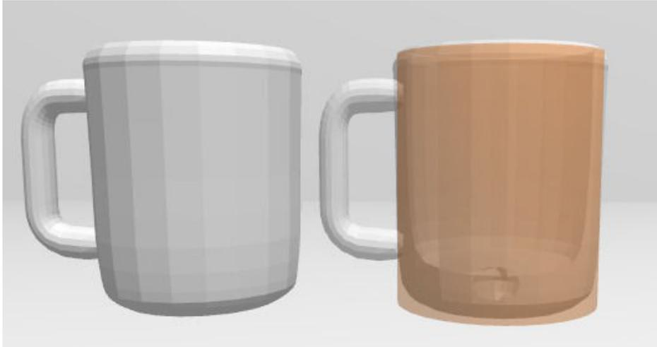
**Fig. 5.9:** RACE cup mesh visual model (left) and cylindrical collision model overlaid (right)
