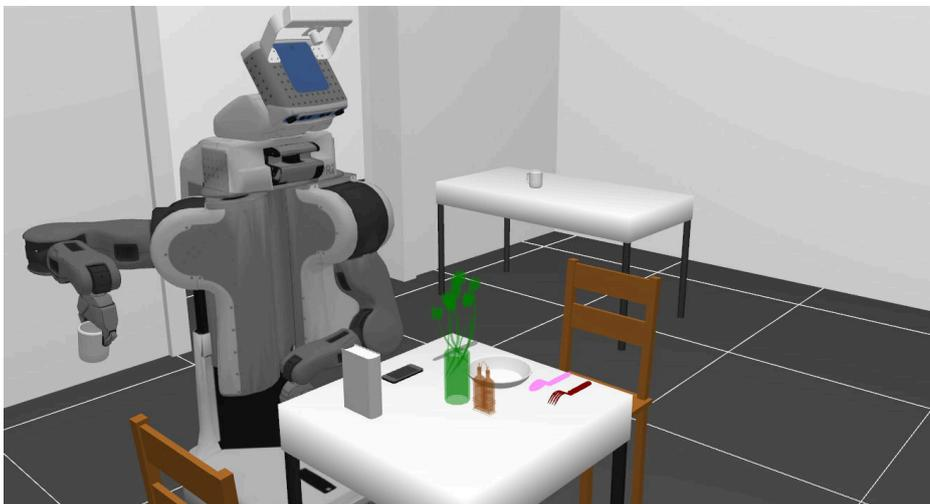
**Fig. 6.8:** The robot reaches the table to place the mug in front of the guest (omitted here, supposed to sit at the side of the table to the robot's left). As the placing area is occupied by various items the robot is unable to succeed.
