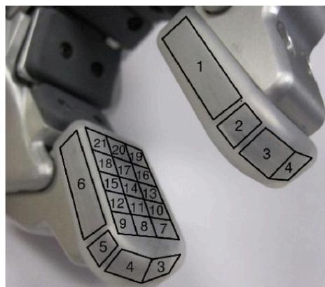
**Fig. 3.2:** PR2 gripper sensors: Arrangement of the 22 pressure sensors on each finger pad.
