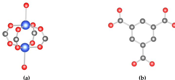
Figure 1.7 – Building units of HKUST-1: (a) the inorganic SBU comprises a copper dimer that is bridged by four carboxylates in an arrangement that resembles the shape of a four-bladed paddle-wheel. The axial positions of the copper atoms within this structure are occupied by solvent molecules that do not contribute to the formation of a framework (b) a trigonal organic SBU that is provided by the btc linker (blue: copper, grey: carbon, red: oxygen, hydrogen atoms are omitted for clarity).
