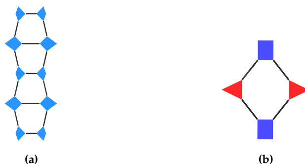
Figure 3.39 – (a) The infinite inorganic SBU of UHM-26 can be abstracted as a ladder-type arrangement of 4-c nodes, shown here in the augmented form (b) the abstracted 4-c paddle wheel motif (blue square) and 3-c organic SBU (red triangle) in their augmented form.
