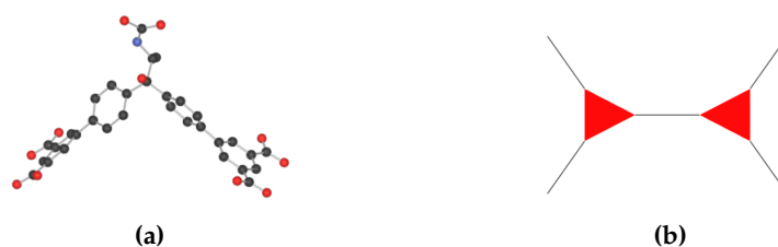
Figure 3.9 – (a) Three-dimensional representation of the linker used to synthesize UHM-25-Ala-Boc and (b) the same linker deconstructed into two three-coordinated nodes shown in the augmented form.
