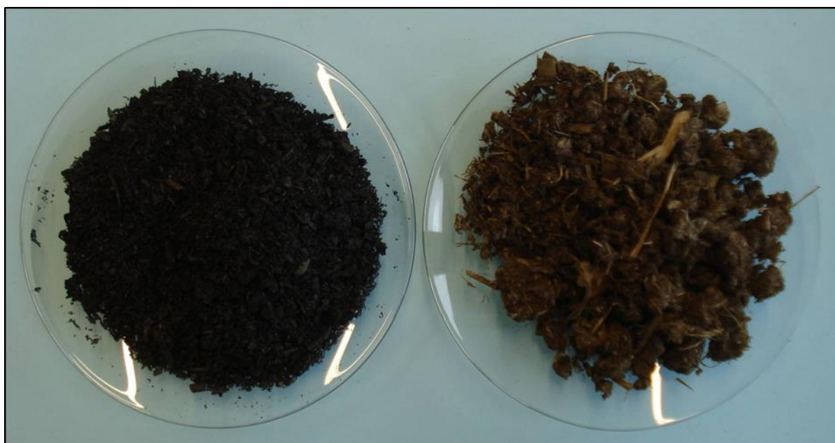
Figure 13: Physical appearance of biochar (left) prepared from dry biogas digestate (right) used as a feedstock; pyrolyzed at 650 °C with a retention time of 30 - 40 minutes.
