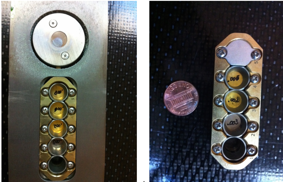
(a) The bottom view of the old photon target (left) and electron scatter foils (right). The greenish powder around the photon target shows the oxidation.
