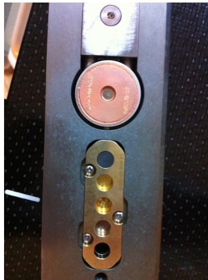
(c) The top view of the new photon target, the electron scatter foil slots, and the carbon target.
