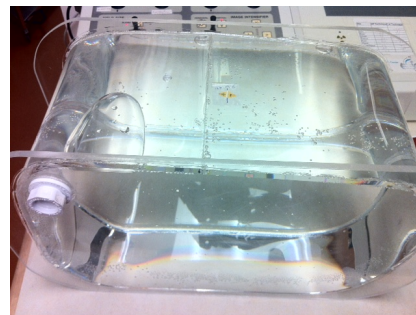
(b) The finished pelvic phantom filled with water.
