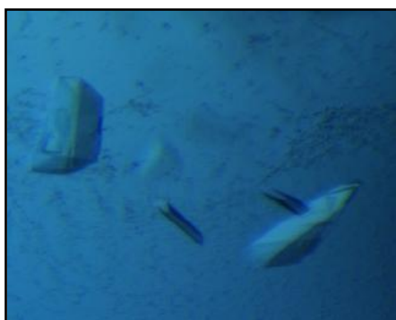
Fig. 17: Low diffracting crystals appeared after one week in condition C6 of the ComPAS suite, consisting of 0.01 calcium chloride, 0.1 sodium acetate pH 4 and 60 % (w/v) MPD in the reservoir. The crystals dimensions varied from 0.18 mm to 0.24 mm.
