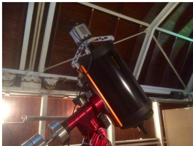
Figure 5.2: The Andor NEO 5.5 on the main focus of the C14.
