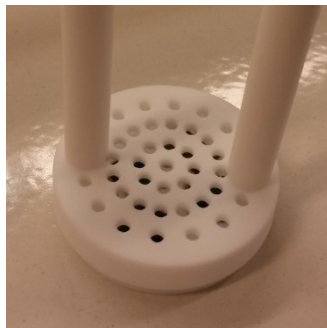
Figure A1.1. Teflon holder for piranha cleaning.
