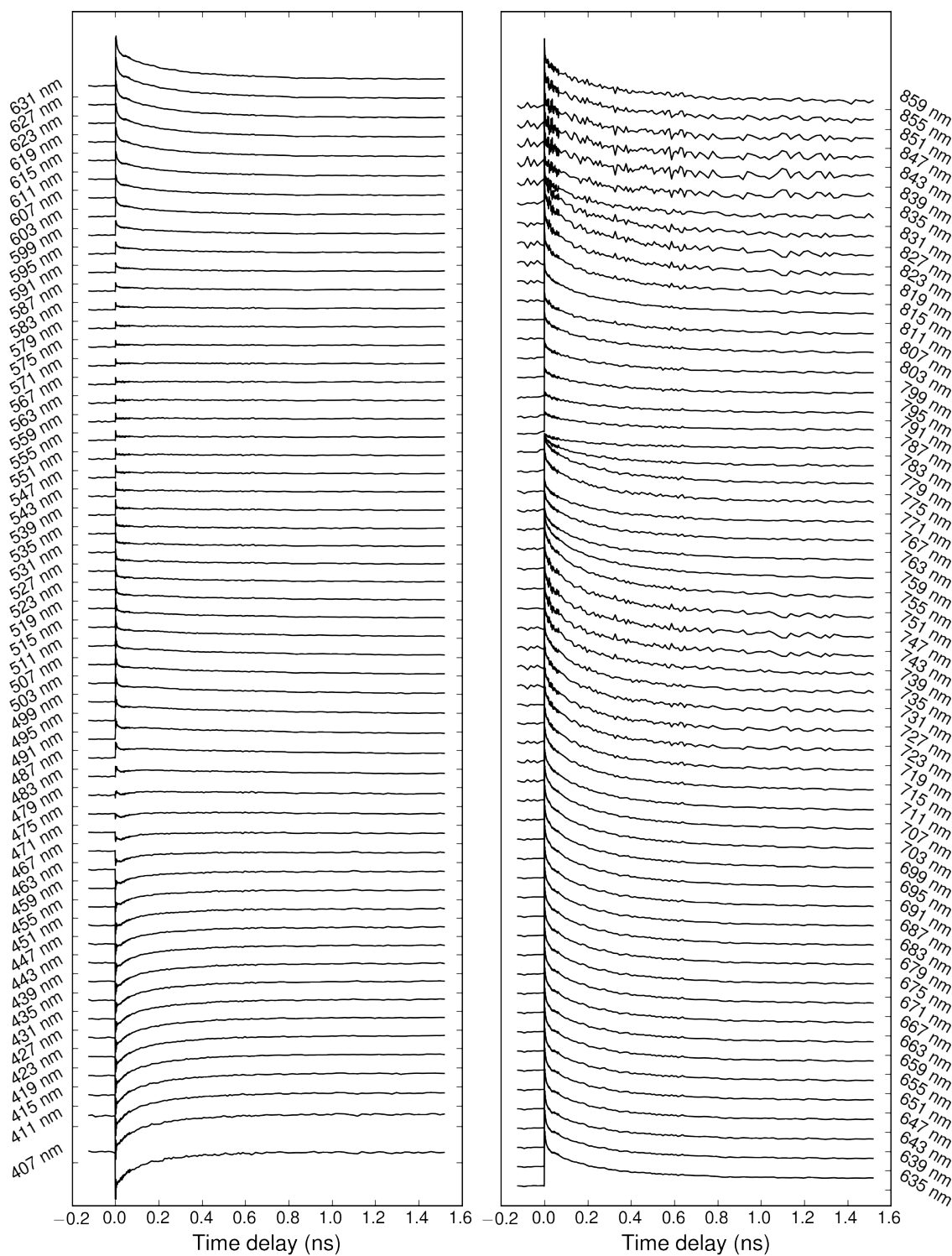
Figure A.5: Wavelength-binned line cuts of the composite dataset taken at 245 K with various time steps of 1 ps, 10 ps and 20 ps after photoexcitation. Each line spans a region of 4 nm, with the center wavelength shown next to each trace. A weak LOESS filter is applied to all traces.
