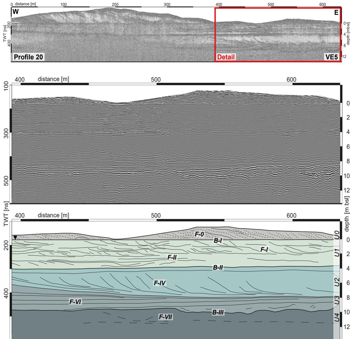
**Fig. 4.4:** Coast-parallel aligned GPR profile 20 comprises of U0 – U4. Overall eastward dipping beds indicate a predominant migration of the barrier towards the east. Foreset packages of U1 represent preserved bottom sets of dunes that migrated into the lagoon.
