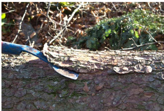
Figure 10: Sampling of Norway spruce bark flakes using a debarking iron
