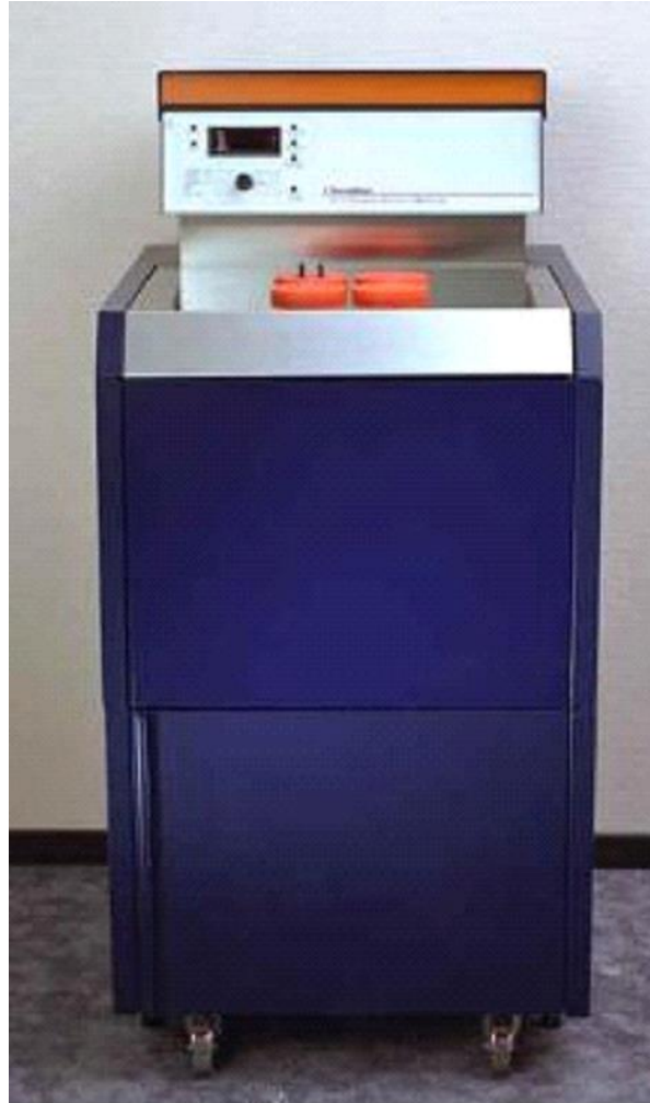
Abb. 1 Das isotherme Wärmeflusskalorimeter 2277 Thermal Activity Monitor (TAM). (Quelle: LKB 2277 Bio Activity Monitor Instruction Manual)
