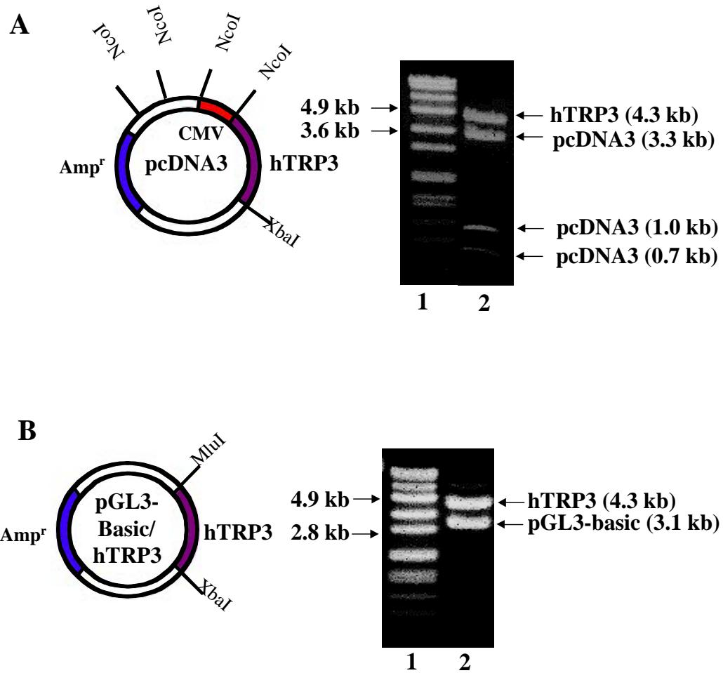
**Figure 1: Restriction enzyme digests of pcDNA3/hTRP3 and pGL3-Basic/hTRP3.** pcDNA3/hTRP3 was digested with NcoI and XbaI. Lane 1 SPP1/EcoRI DNA molecular weight markers. Lane 2 pcDNA3/hTRP3 cut with NcoI and XbaI (A). pGL3-Basic/hTRP3 was digested with MluI and XbaI. Lane 1 SPP1/EcoRI DNA molecular weight markers. Lane 2 pGL3-Basic/hTRP3 cut with MluI and XbaI (B).
