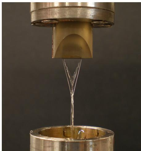
**Figure 4.2:** The sapphire nozzle produces a liquid flat sheet jet of 100  $\mu\text{m}$  thickness over a width of about 6 mm. The sheet flows downwards at an adjustable speed in the range of 0.5 m/s to 30 m/s (in this photo:  $\sim 5$  m/s).
