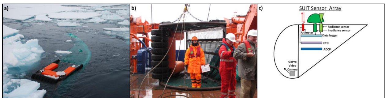
Figure 1. The Surface and Under-Ice Trawl (SUIT): a) in the water being towed by the RV Polatstern; b) laying on its side on the deck of the Polatstern; and c) depicted in a simplified diagram showing a side view with mounted locations of the sensors (not to scale).
