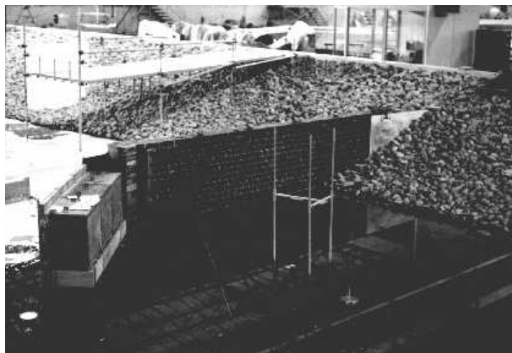
Figure 45: Wall construction: prevents waves coming from behind the wall, creating a wave shadow zone.
