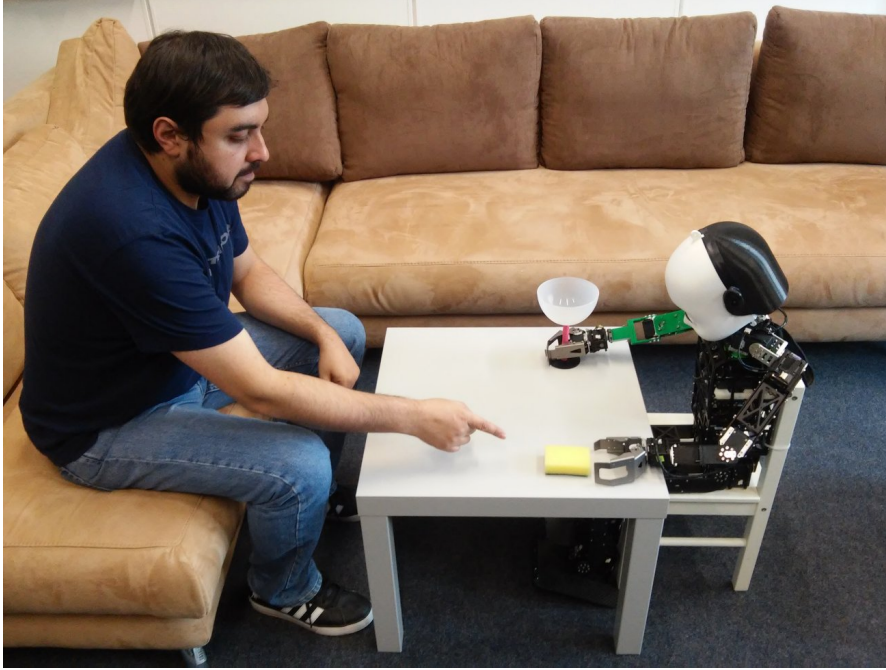
Figure 2.5: A scenario with human-robot interaction where the apprentice robot is supported by a parent-like trainer to complete the task.
