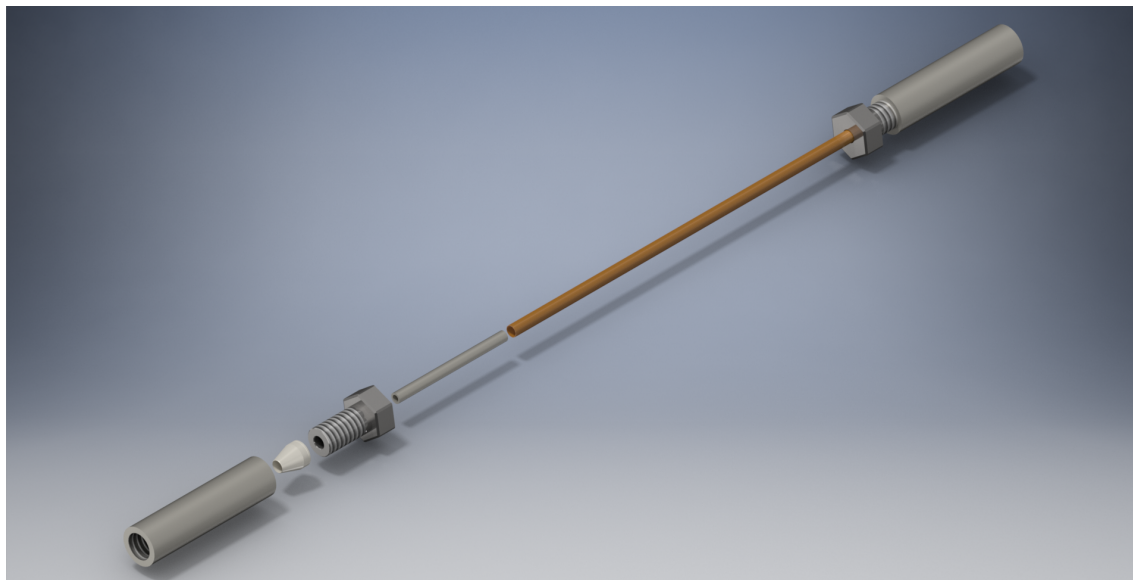
Figure 4.9.: Exploded 3D rendering of the X-ray flow cell based on commercially available Kapton tubing.
