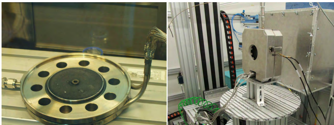
Figure 4.4: Left: Bottom body part of FlexiStore, filled with a sodium alanate pellet. Right: Complete FlexiStore setup with attached thermal insulation, hydrogen supply and thermocouples before an in situ Neutron Radiography measurement at NECTAR. The tank is mounted on the rotational unit in front of the scintillator.
