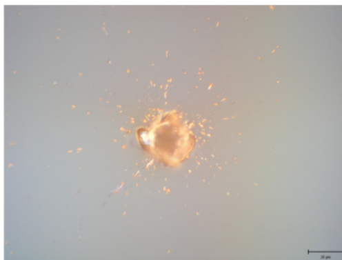
Fig. 7.11.: Marker on the map of amorphous carbon sample with 890 nm thickness, exposed to single shots at FLASH 2008 with 177 eV . Scale size on the bottom right side is 20 \mu m .
