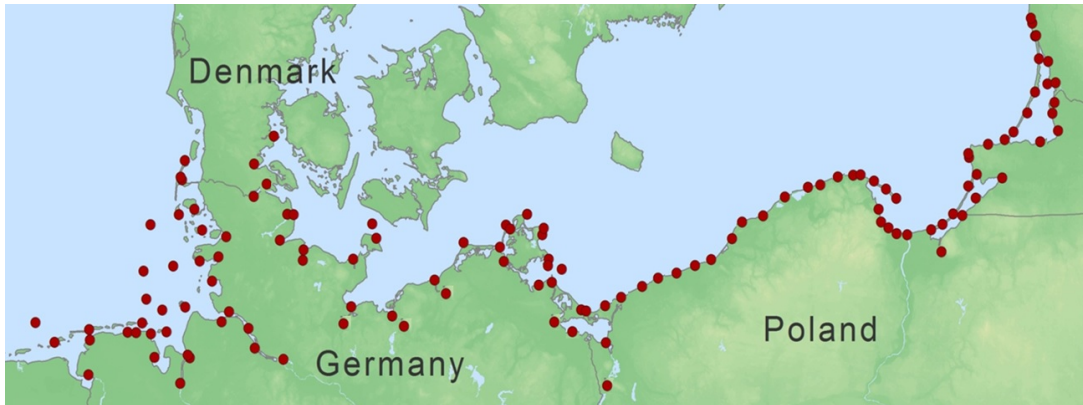
Figure 2.2.: Positions of all 164 signal stations with weather observations from 1877 to 1999 along the coastline of the German Bight and the southern Baltic Sea. Not all stations existed during the same time period.
