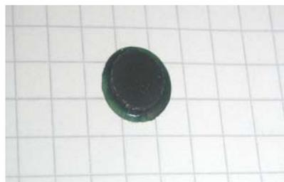
Figure 10-5. Electrode-membrane assembly of s-PEEK·ZrO<sub>2</sub>·MoPA (64·8·28) for proton conductivity measurements.
