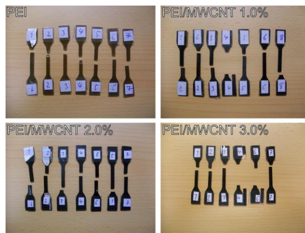
Figure 117: Photographs of the broken samples for tensile testing of PEI and PEI/MWCNT with 1.0 wt%, 2.0 wt% and 3.0 wt%. All samples showed brittle fracturing behaviour with a few samples breaking at two points.
