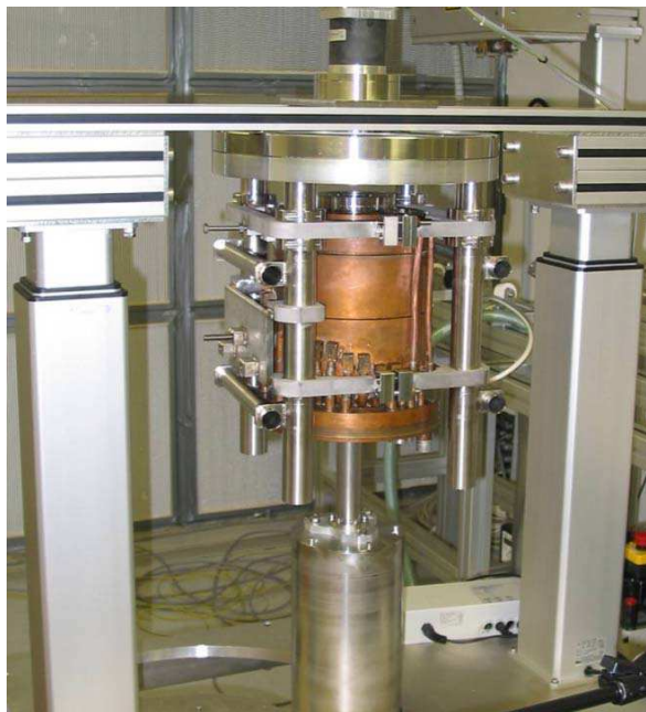
Figure 4.43: Vertical cleaning set-up for gun cavities [70].
