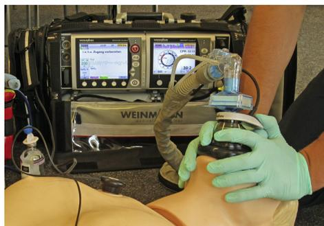
**Figure 1.** The prototype device (Defikom<sup>TM</sup>, WEINMANN Emergency Medical Technology; Hamburg, Germany) with the switch for triggering ventilations via the face mask (MEDUtrigger<sup>TM</sup>, WEINMANN Emergency Medical Technology) in the foreground.
