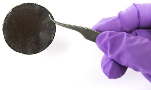
Figure 4.4: Picture of the graphite oxide membrane procured from Graphenea S.A.
