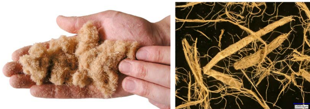
Figure 1.4 Visual (left) and microscopic (right) image of MDF fibers and fiber bundles obtained after defibration.
