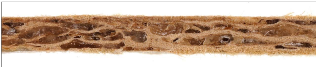
Figure 6.5 Panel cross section manufactured from a compound produced by the up-scaling process containing a 50/50 ratio of wood fibers to polymer.
