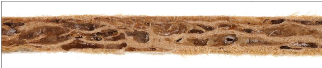
Figure 5.4.5 Wood fiber compound (50/50) manufactured to panels. Here view on the cross section.
