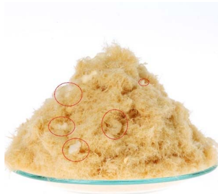
Figure 6.3 Obtained compound after simultaneous defibration and compounding (Chapter 5.4). The red circles show larger polymer fragments.
