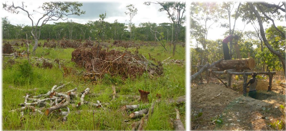
Fig. 17 Cutting planks in a pit saw dug on site
