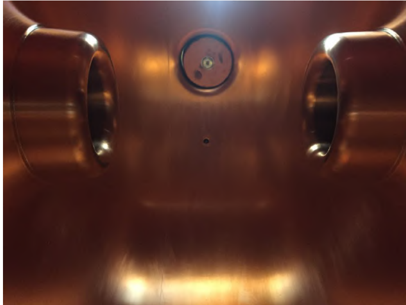
FIGURE 3.4: The photo of the inner surface inside the cavity. The surface is polished to maintain the high electromagnetic reflection, one can see the two nose cones preserved for the beam line.
