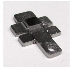
Figure II.23: Ir single crystal fixed on a W plate.
