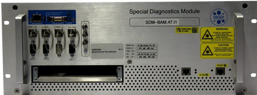
Figure 3.6: Front view photograph of the new BAM electro-optical unit.
