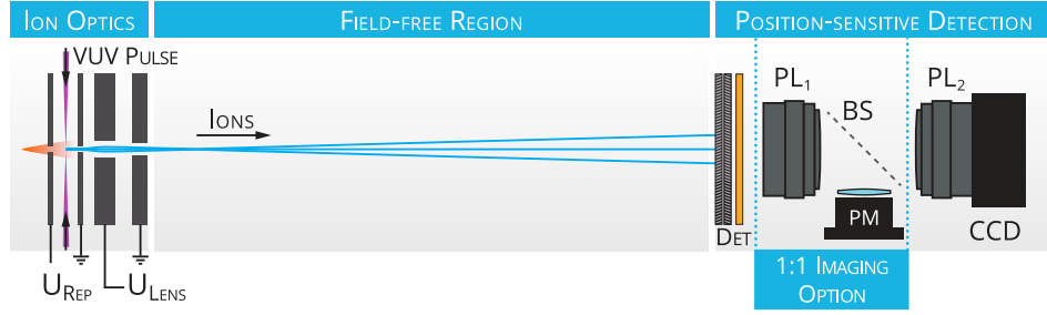
FIGURE 3.5 – Schematic overview of the ion image apparatus. The apparatus is divided into three parts: (a) The ion optics part comprising the electrostatic lenses. (b) The field-free region, where ion are separated depending on mass-to-charge ratio. (c) The position sensitive detection, where the MCP/phosphor screen detector can be imaged by a CCD camera in two imaging geometries.
