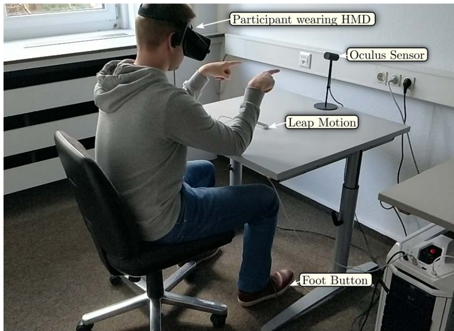
Figure 4.26: Illustration of the experiment setup.
