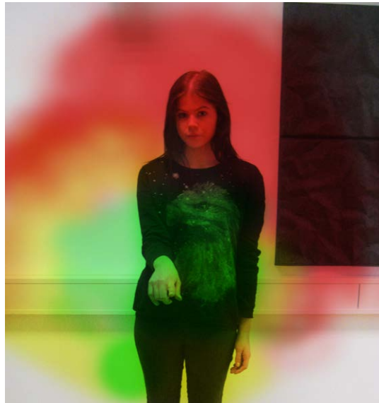
Figure 4.3: Heatmap illustration of comfortable and uncomfortable poses; red regions were evaluated as uncomfortable, green regions as comfortable poses.
