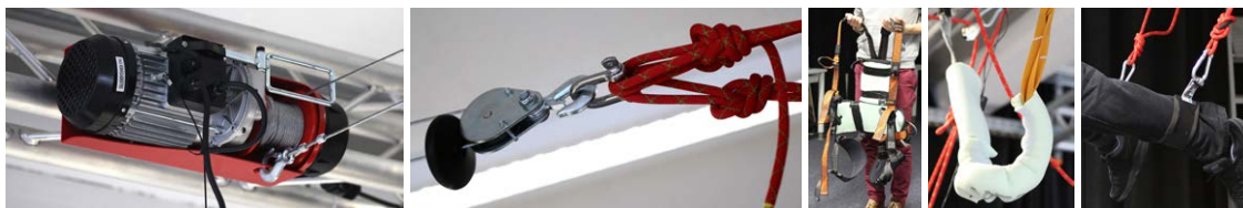
Figure 5.7: Components of the mounting system. From left to right, there is the motor winch mounted horizontally at on the truss, the connection between the carabiner of the winch and the climbing ropes, the climbing harness, the Thera-Band sling for load reduction at the chest and the fixation straps at the ankles.
