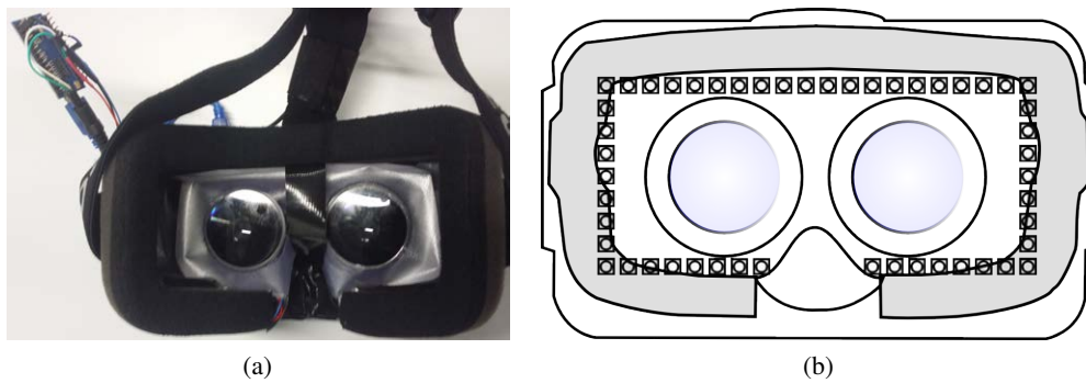
Figure 5.27: a) The Oculus Rift DK2 with peripheral display extension prototype and diffusing foil. b) Schematic illustrating the LED placement.
