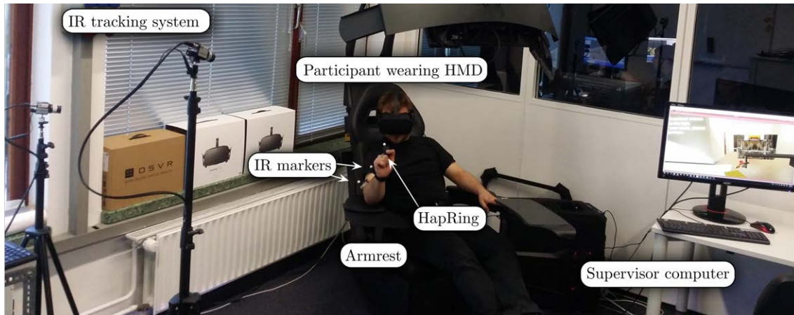
Figure 4.15: Illustration of the confirmatory study setup.
