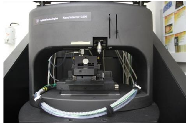
Figure 16: Agilent G200 nanoindenter, with zoom on its sample stage
