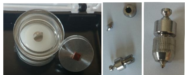
Figure g: left – diamond tip and polished Copper on the aluminium sample holder; middle and right – tip-holder.
