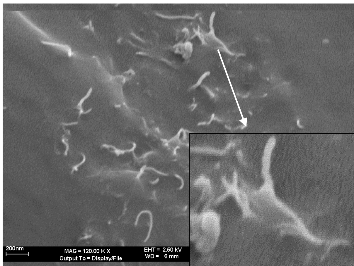
Fig. 66: SEM picture (magnification 120,000 times) of an sPP/MWNT nanocomposite containing 0.9 % of carbon nanotubes (KW323).
