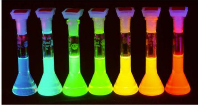
Figure 13. Continuously shifting the emission of CdSe nanoparticles (passivated with a ZnS shell) from red to blue by reducing the size of the particles and increasing the bandgap. The figure was adopted from 64 .
