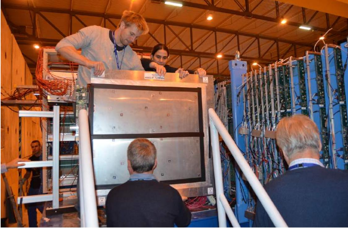
Figure 12.1: W-DHCAL in tungsten stack with the tail catcher during installation of the AHCAL layer at the H8 SPS beam line at CERN.
