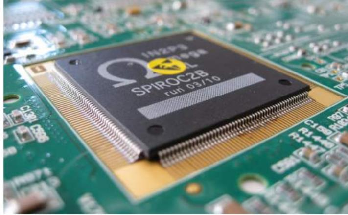
Figure 6.4: The Spiroc2b readout chip, a dedicated very front end readout chip designed by Omega [63]. The chip is hosted in a low profile casing. A ditch in the PCB of the HBU lowers the overall height of the HBU to 5.4 mm.
