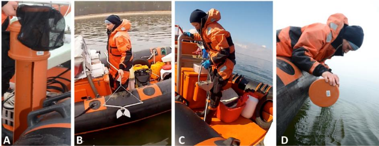
Figure 2: Field sampling procedure, using the Van Veen grabber from a zodiac. (A) a mesh bag is mounted on the open side of the washing tube (with longitudinal opening on the left), (B) the van Veen grabber, held by hand, prior to sampling, (C) the van Veen grabber with the plant sample inside the bucket, (D) after the grabber content was put into the washing tube, the sample was washed to remove sand particles.
