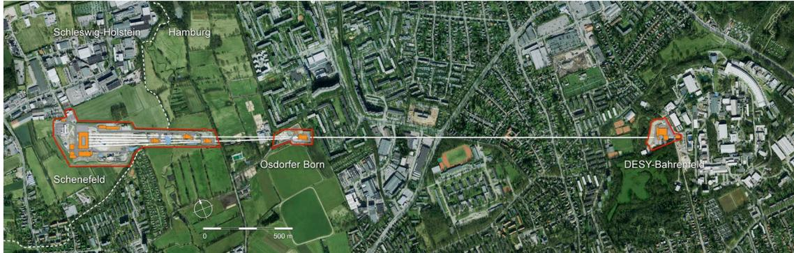
Figure 2.2: The European XFEL X-ray laser is a 3.4-km-long facility which runs essentially underground. The three sites (framed in red) are located in Hamburg (DESY-Bahrenfeld and Osdorfer Born) as well as in the south of the city of Schenefeld (Pinneberg district, Schleswig-Holstein). - Copyright European XFEL / FHH, Landesbetrieb Geoinf. und Vermessung, [5].
