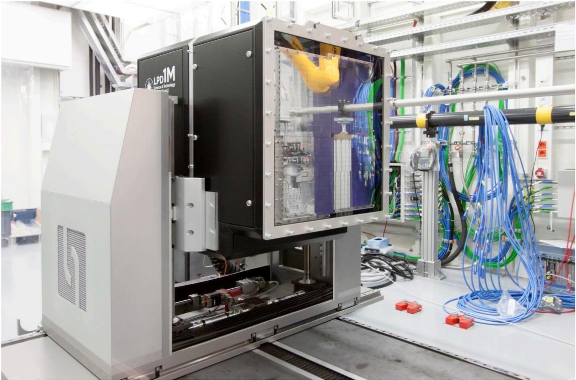
Figure 2.12: The Large Pixel Detector in its final location as part of the FXE instrument. Copyright European XFEL, [5].
