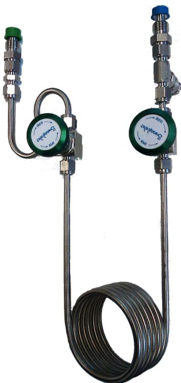
**Figure 4.5.:** “Trap No3”, consisting of 180 cm stainless steel tube with 4 mm inner diameter, loaded with 10 g of activated charcoal. This trap will be used in the final separation line and labelled “AC1”.
