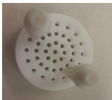
Figure 1: Teflon holder used for the piranha cleaning
