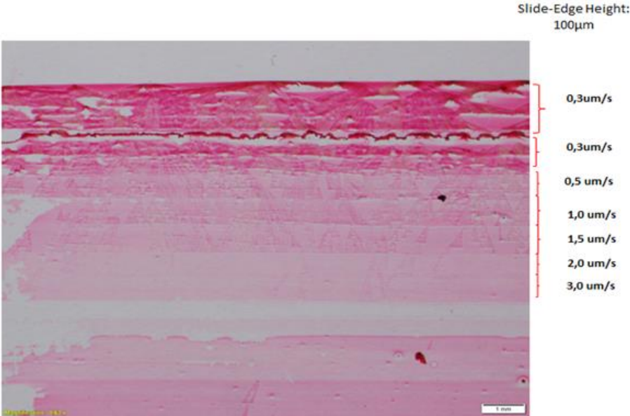
Figure 2.13: Crystallization on the edge with a water solution 5 mg/mL and a constant solution supply rate held at 0.03 mL/hour
