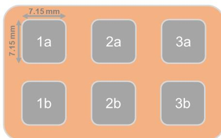
**Figure 14: Experiment PIRL optimization III – three different laser pulse energies for defining optimized laser parameter for preferably thinnest ablation deepness.** Adjusted pulse energies (1a&1b) 144  $\mu$ J; (2a&2b) 166  $\mu$ J; (3a&3b) 184  $\mu$ J.
