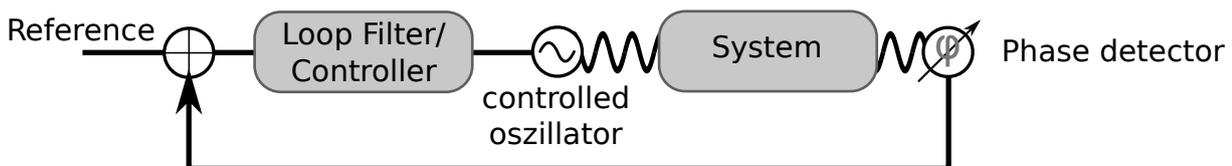
**Figure 9.8:** Components of a phase locked loop.
