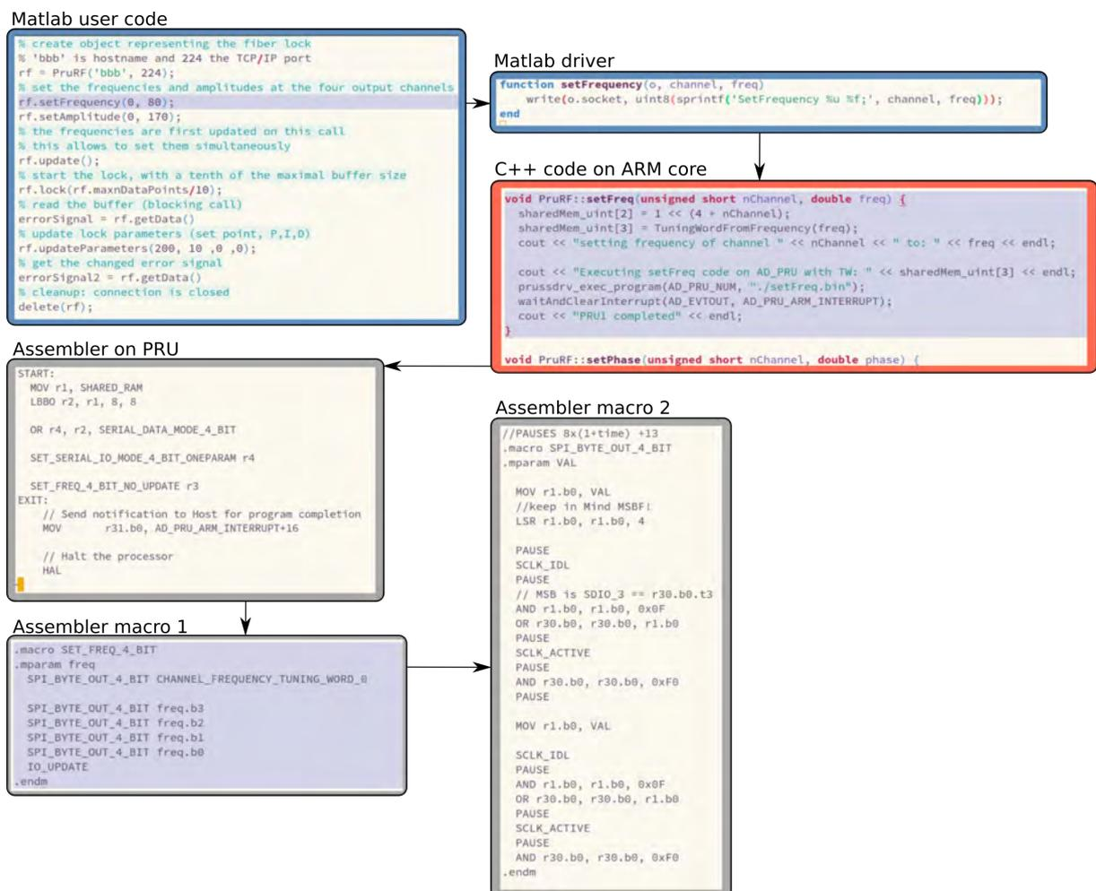
Figure C.3: Code snippets for a simple command to set the frequency of the lock.
