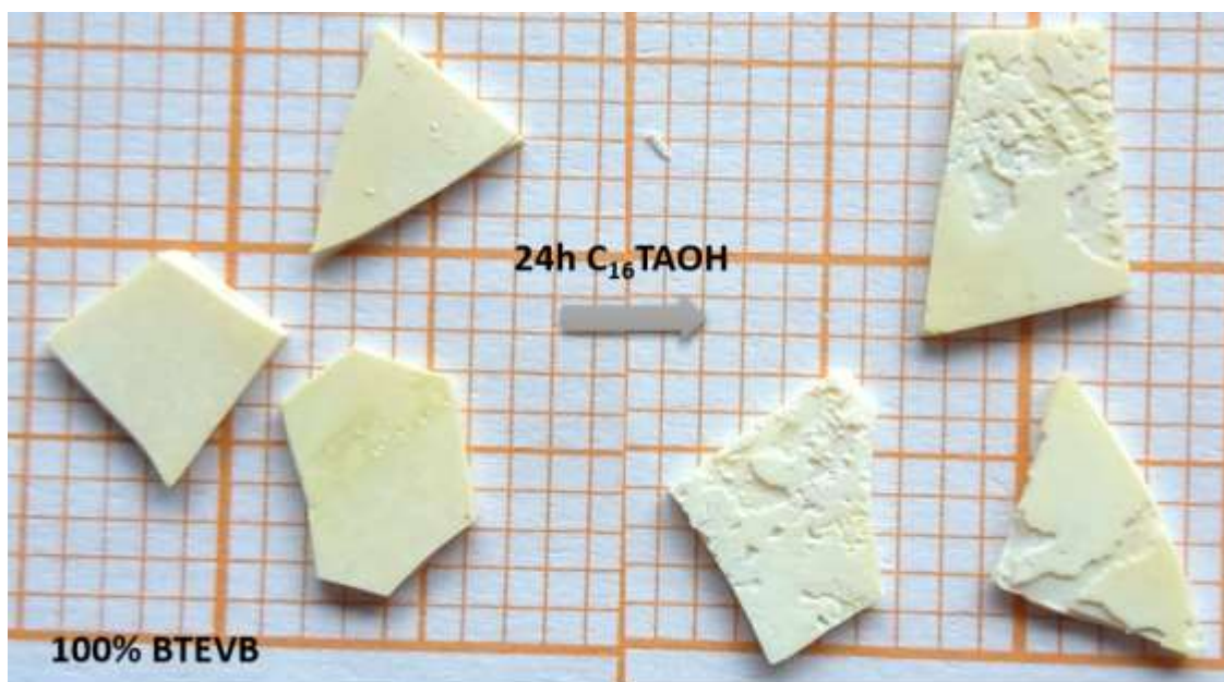
Figure 4-144: Photos of the CPG membrane impregnated with 100 % BTEVB and the respective sample after pseudomorphic transformation in C_{16} TAOH for 24 hours. The background is plotting paper with 10x10 mm bold squares.
