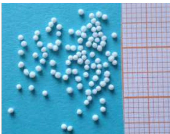
Figure 4-151: Photograph of the \text{SiO}_2 beads that were obtained by templating with alginate hydrogels. Plotting paper with 2 \times 2 \text{ mm} squares on the side is the scale bar.
