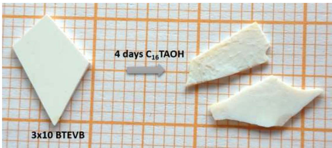
Figure 4-143: Photographs of the CPG membrane impregnated with 3x10BTEVB and the respective sample after pseudomorphic transformation in C_{16} TAOH for four days. The background is plotting paper with 2 x 2 mm squares.
