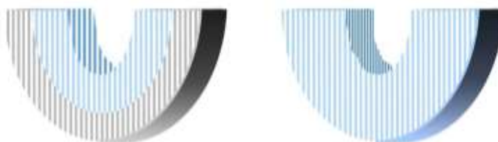
Figure 4-133: Two different structures of the organosilica (blue)/silica (gray) hybrid materials are in accordance with the results from different characterization methods. It is either one pore system of mixed organosilica/silica species or it consists of two phase, a mixed phase (light blue) and a pure silica phase.
