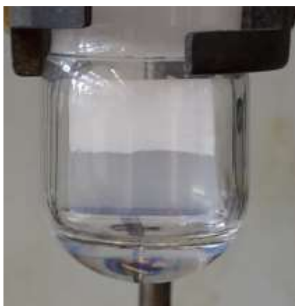
Figure 8-1: Photograph of the setup for the impregnation of a CPG membrane with a BTEVB-containing toluene solution.
