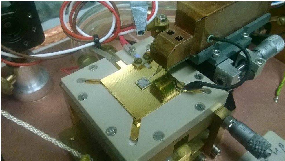
FIGURE 4.14: A diamond sensor is in the opened "beta-setup" box before the measurement. The needle is on top of the diamond sensor, which is mounted in the center of the high voltage golden plate. The black hole in an iron pyramid is a dry-air source (5% oxygen + 95% dry nitrogen). During the measurement, this scheme is covered with a black wooden box. Inside on top, the box has two mounted layers of scintillation detectors.
