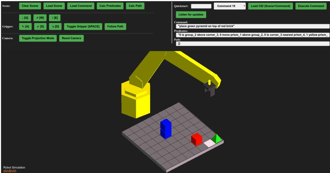
Figure 4.12: Screenshot of the web-based simulator. It can be controlled by the user (buttons on the left side) and scenes from the data set can be loaded (right side). The simulator can also be controlled via an API to be able to connect it to our bidirectional processing chain.
