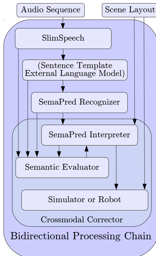
Figure 4.14: The architecture of the bidirectional processing chain.
