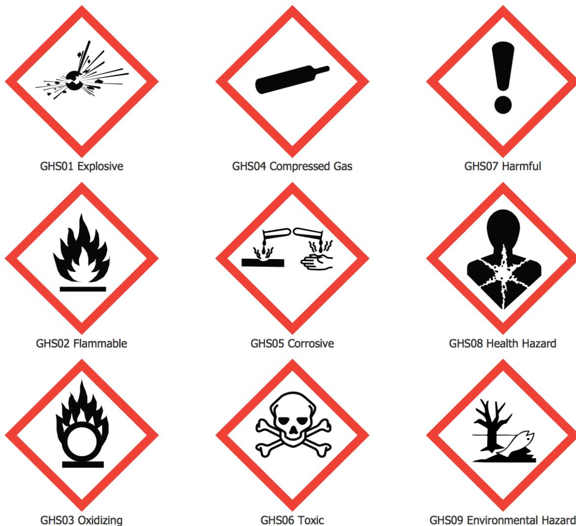
**Figure 5.1.1: Hazard Pictograms according to GHS.** Diagram adapted from [357].
