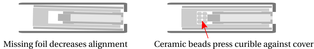
Figure 5.31.: Removing the tantalum foil can cause a misalignment of the inner oven parts. This can be countered by pressing the tip of the crucible against the oven cover.
