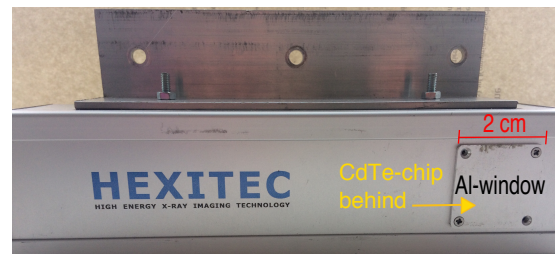
Figure 2.11: Photograph of a HEXITEC detector. The active area of 4 \text{ cm}^2 is covered by an Al-window located at the right side of the module.
