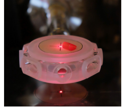
Figure 4.5: The new glass science cell. Shown is the glass cell after integration into the experiment after the surrounding coils and breadboards were reinstalled. The paper sheet was used to align the pilot beam which is both central and orthogonal to both upper and lower glass cell windows and is used for the subsequent microscope alignment.
