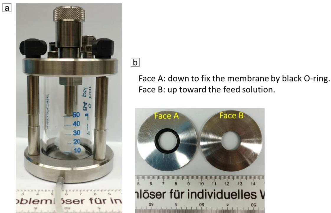
Figure 3.3. (a) A photo of the employed EMD Millipore XFUF04701 cell, (b) Photos of the in-house prepared reduction ring to reduce the effective membrane size.
